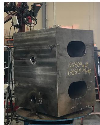
**TOP:** 18-5M Type 52 BOP Lower Housing; weld prep completed to mount weld neck flange
